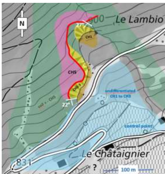
Fig. 3 Geological map of CH and immediate surroundings. The red line represents the thin CH4 unit. Circles are control points. 1918 swisstopo base.
