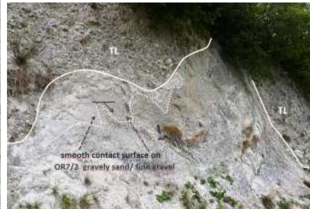
FIGURE 75 Smooth TL-OR7/2 contact surface.
