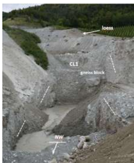
Fig. 27 Northerly dip of the CL1 DFD within the CL trench. Gneiss boulder ~3 m wide.
