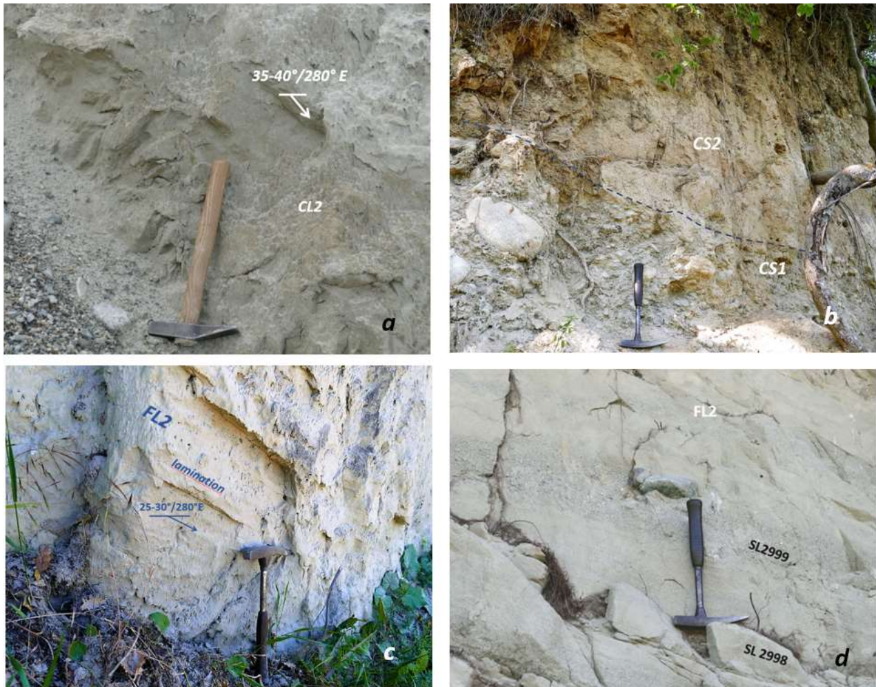
Fig. 40 Examples of laminated CL2, CS2 and FL2 sand ( a , c and d ), with parallel gravel streak in ( d ) and in clear contact with CS1 in ( b ).
